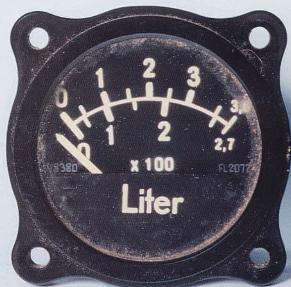
Dual fuel tank contents gauge.
