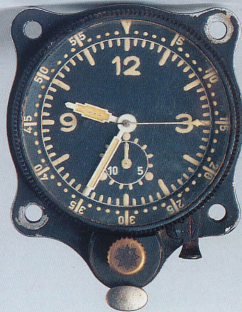
Chronometer fitted with stop watch button.
