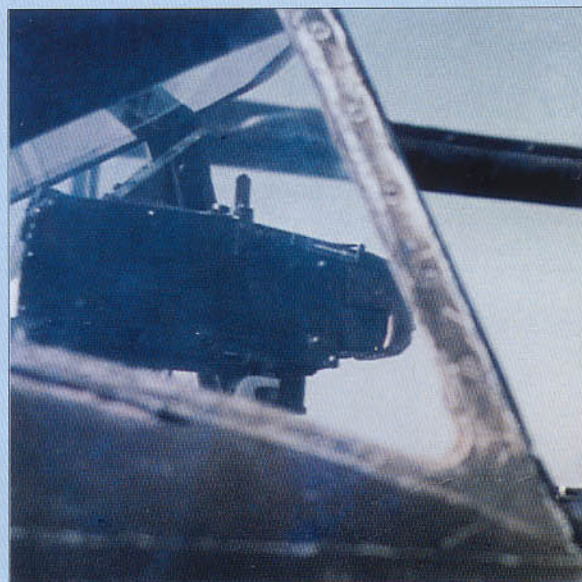
Above: The EZ 42/1-A1 gyroscopic gunsight (EZ - Einheitszielvorrichtung / Standard sighting device), manufactured by Askania, was introduced late in 1944 and intended for fighters such as the Ta 152, BV 155 and the Me 262 (shown above).
