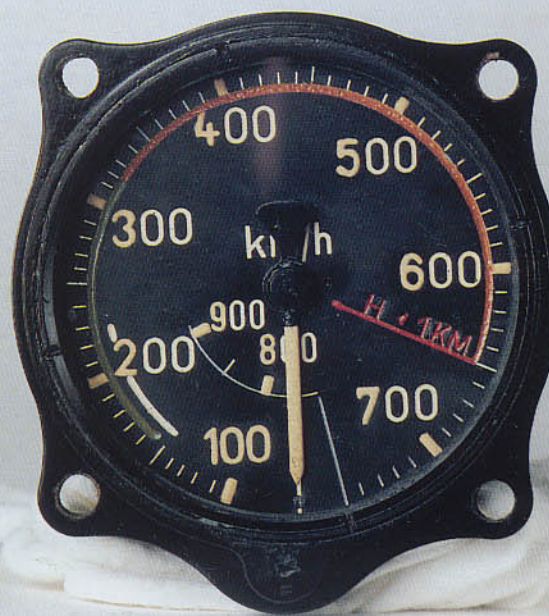
Air speed indicator calibrated to 600 km/h.
