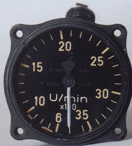
Original Bruhn tachometer calibrated to 3500 rpm.
