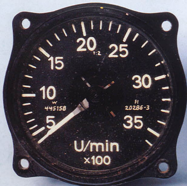
Tachometer calibrated to 3500 rpm.
