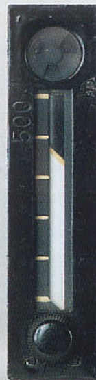
Ammunition round counter (left) + armament instrument.
