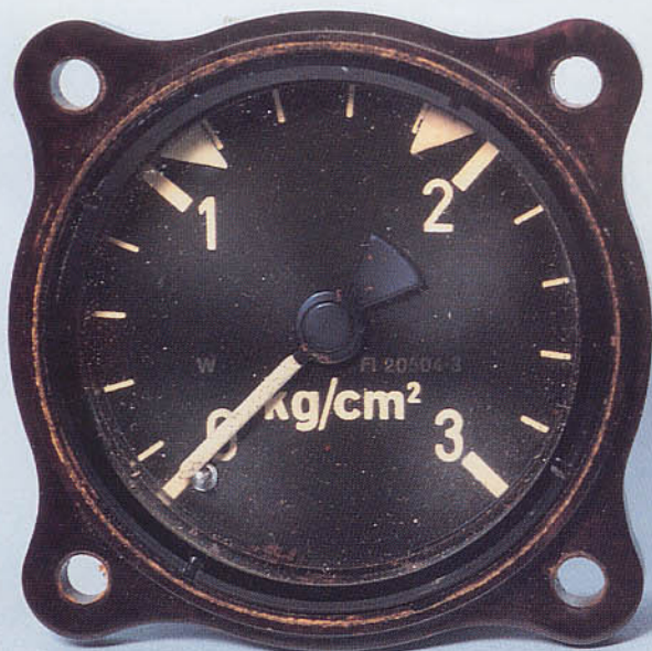
Methane/water boost pressure gauge.
