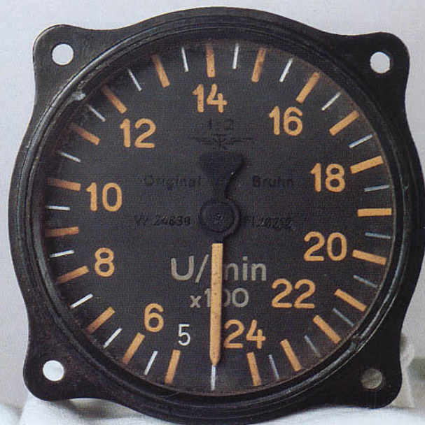
Tachometer calibrated to 2400 rpm marked Original Bruhn.
