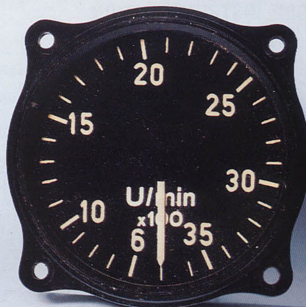
Tachometer calibrated to 3500 rpm.
