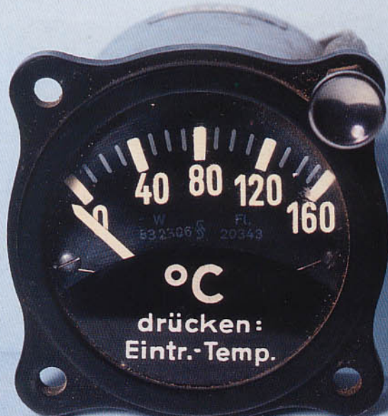
Supercharger outside air intake temperature, Siemens.
