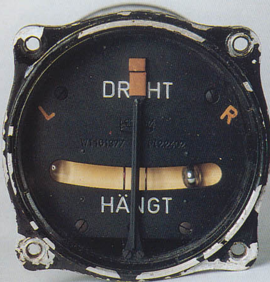
Turn and bank indicator made by Askania.
