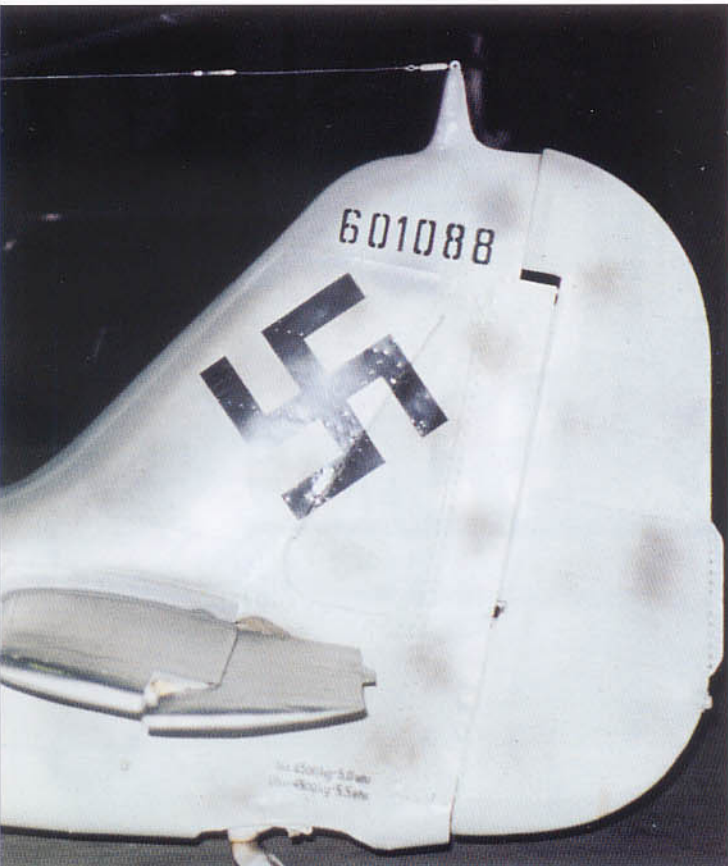
Above and below: Apart from a narrow filler section (17 below), the all-metal tail assembly for the Fw 190 D-9 was identical to that used for all of the Fw 190 A-series. The photograph above is a close-up of the D-9 on display at the Air Force Museum at Wright-Field.
