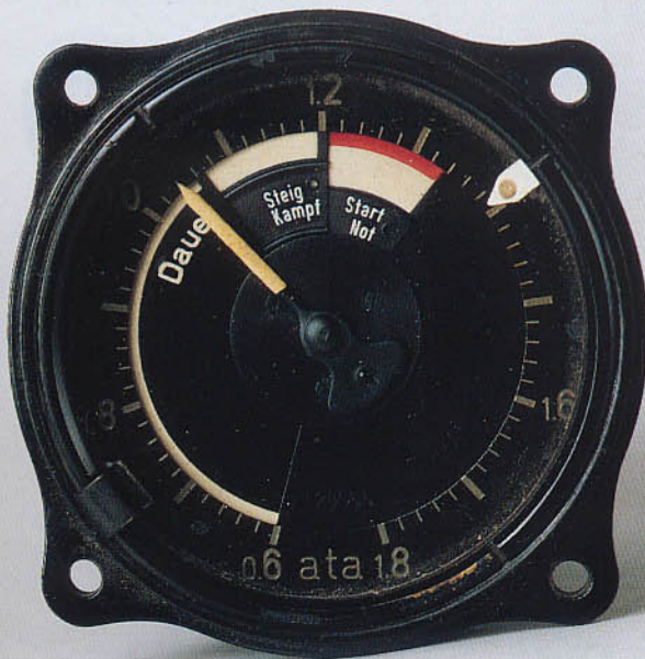
Manifold pressure gauge marked for combat power + restart.
