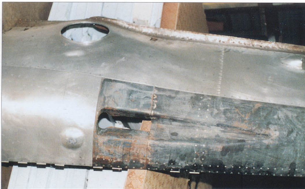
Right: A close-up of the top of the starboard cowl stripped of all paint and ready for final refinishing. Note the elongated opening for the cowl-mounted MG 131 machine gun and the piano hinge running along much of the top centerline.
