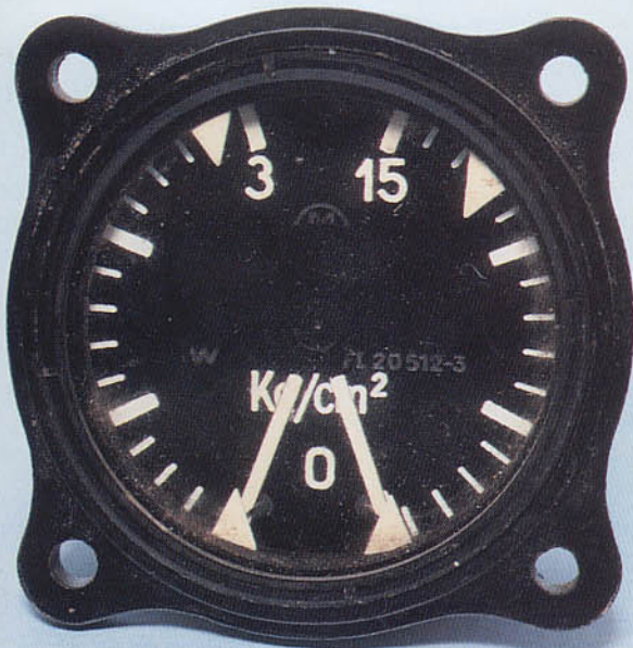
Dual fuel and oil pressure gauge.
