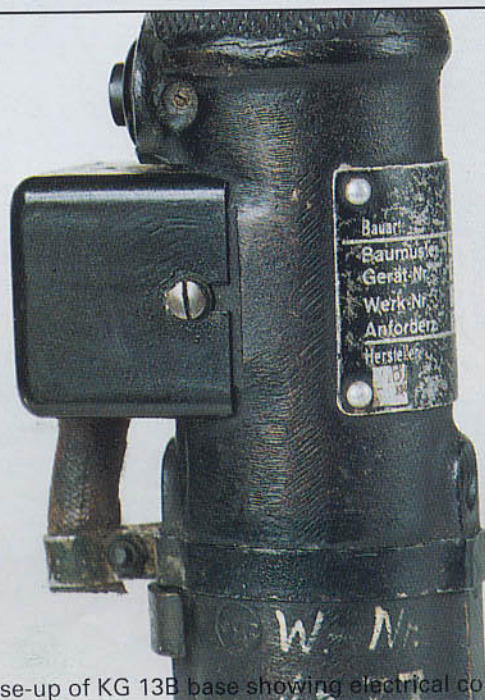
Port side view of Bauart made KG 13B control column.
