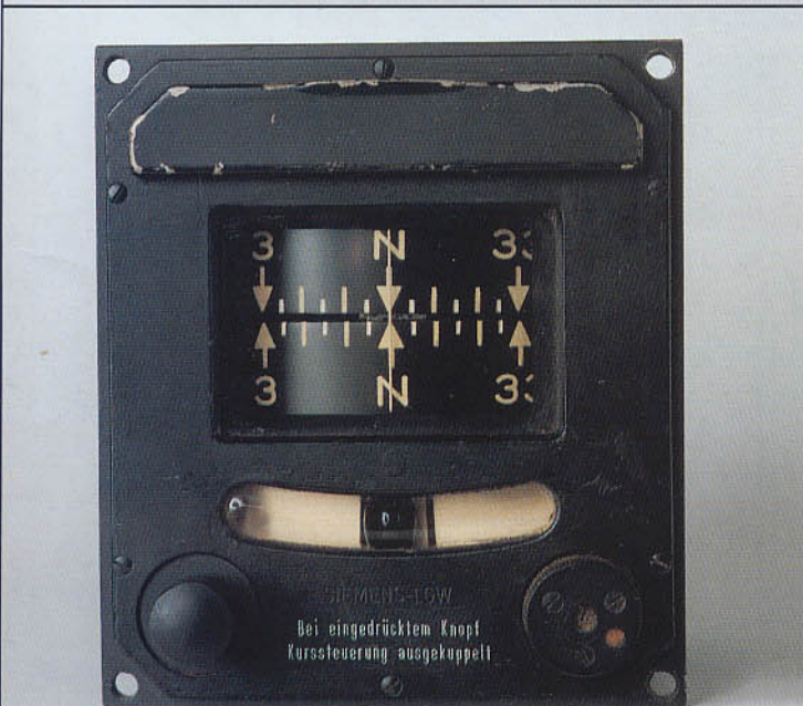
Siemens-Low combined coarse repeater + slip indicator.
