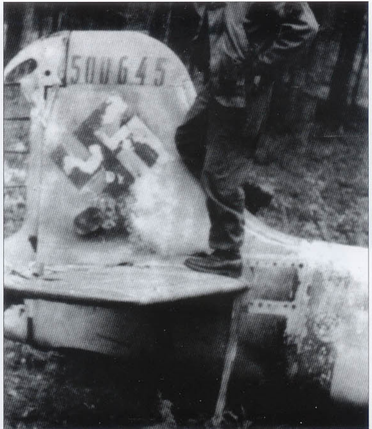
Above and below: During the last half of 1944, the German aviation industry made use of the woodworking shops throughout Germany to create numerous parts and whole assemblies from wood such as the optional wooden tail assembly shown above on Fw 190 D-9, W.Nr. 500645.
