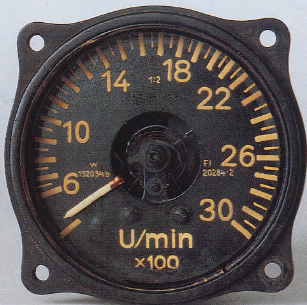
Tachometer calibrated to 3000 rpm made by Deuta-Morell.
