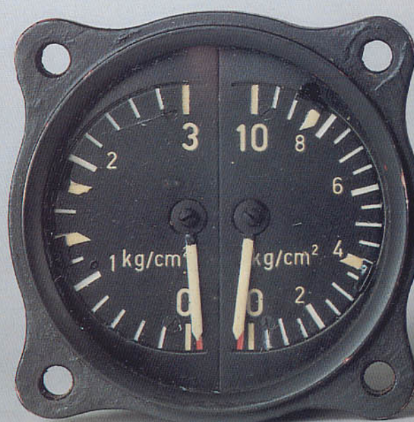
Dual fuel and oil pressure gauge.
