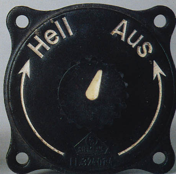
Dimmer control made by Siemens.
