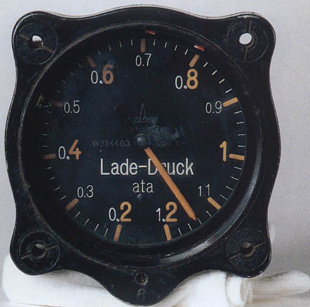
Manifold pressure gauge made by Askania.
